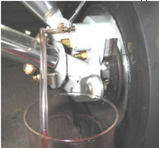
Figure 43 Bleed Drain Hose Connected
