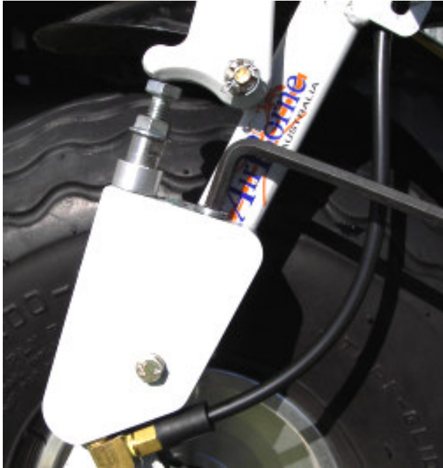
Figure 38 Remove Reservoir Plug
