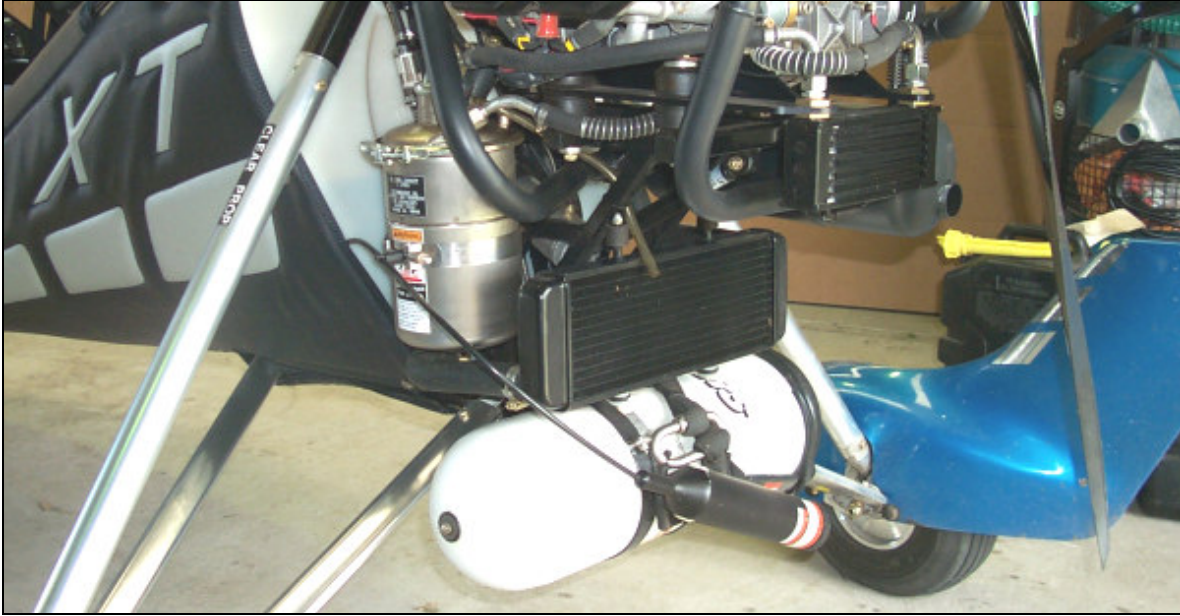
Figure 76 Ballistic Parachute Installation, XT-912
