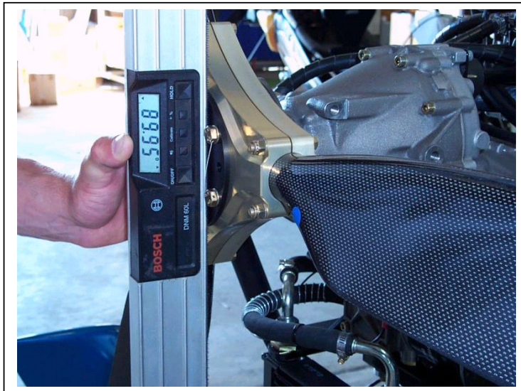
Figure 68 Prop Hub at 89.95 Degrees After Correct Shimming of Front Wheel
