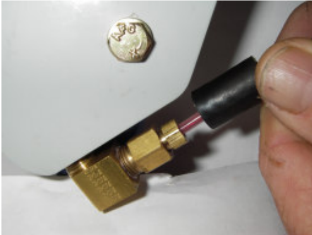
Figure 41 Master Cylinder, Push Triple Sleeving Over the Compression Fitting Nut
