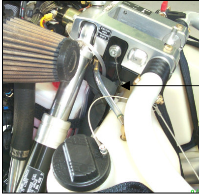
Figure 83 Side View, Bridle Attachment
