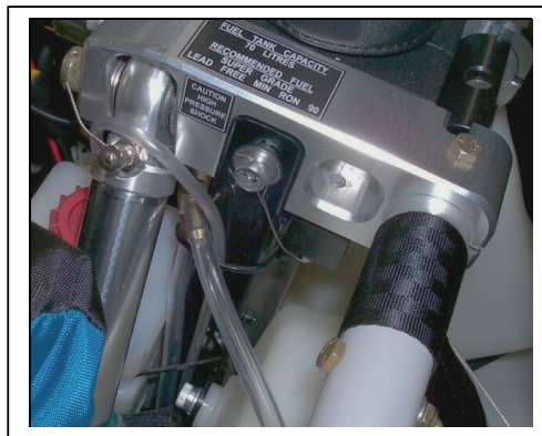
Figure 56 Rear Landing Gear and Engine Mount Attachment to Mast Block
