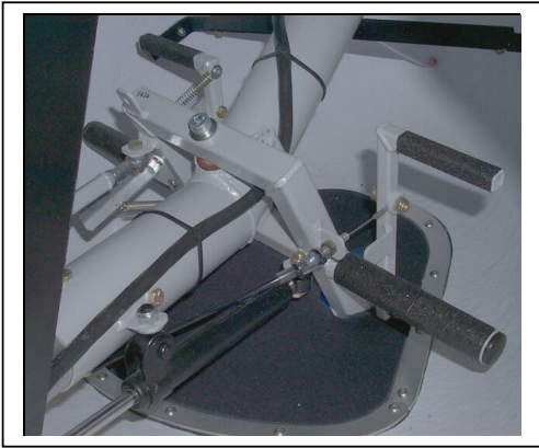
Figure 54 Front Landing Gear Attachment
