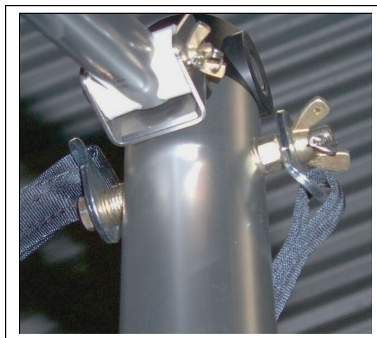
Figure 24 Mast Top Safetying
