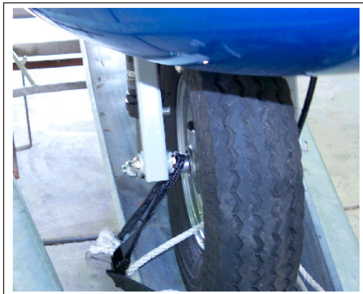
Figure 10 Front Wheel Tie Down
