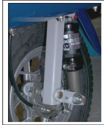
Figure 55 Front Fork to Wheel Attachment
