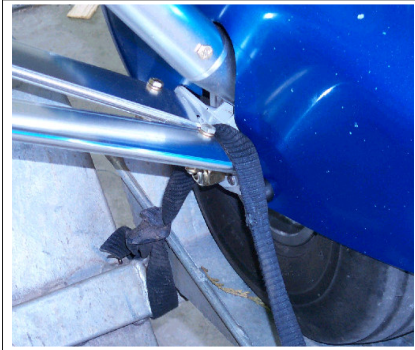
Figure 11 Rear Wheel Tie Down
