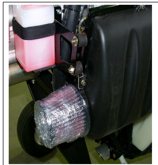
Figure 16 Air filter Protection During Cleaning
