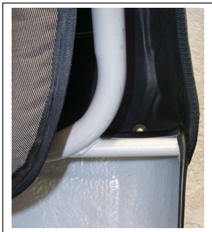
Figure 59 Pod Attachment to Seat Frame
